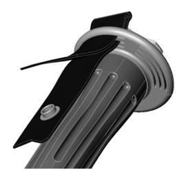
Weave the end of the strap down and back up through the slots in the flange of the handle. The strap may be pulled through the slots to adjust for size.
