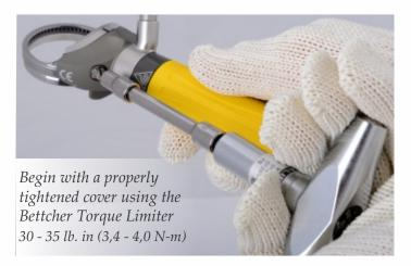
The "best practice" to secure the pinon cover and housing is to use a torque limiting T-handle tool (Bettcher Part #183898) to secure the housing quickly and properly.
