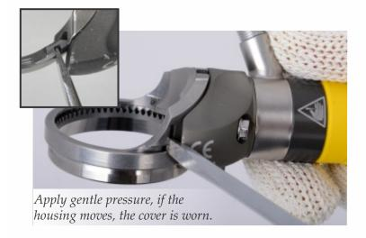
Using a straight-blade screwdriver, slowly apply pressure to the housing. If the housing moves easily without much pressure, the cover is worn. It should be replaced, as it can no longer secure the blade and housing and may become a safety issue in addition to running rough.
