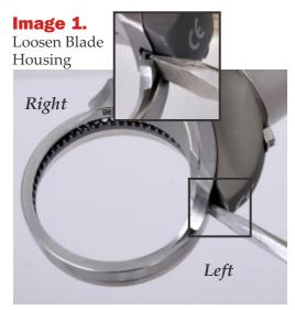
If the blade is not moving freely, loosen the left screw and gently pry the housing open.
