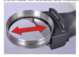
The blade should turn freely with a slight amount of clearance in the direction shown by the arrow.
