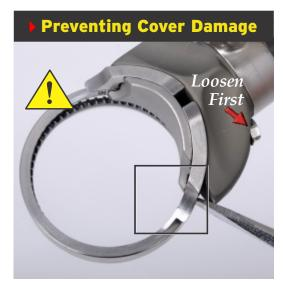
Damage occurs when the housing is pried without first loosening the cover screw (red arrow).
