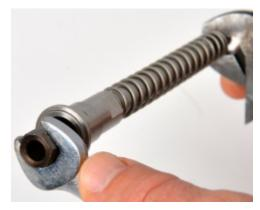
Place the Drive Shaft Tool over the square-end of the driver shaft fits into the square hole of the tool. This is a left-hand thread, so turn clockwise to loosen.
