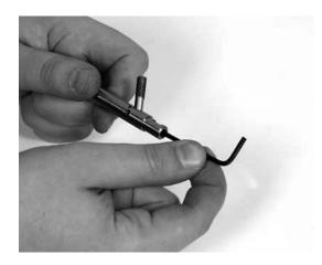
• Slide the steeling rod shaft through the locator and into the rod mount. Tighten the steeling rod screw.
