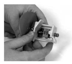
• Install the steeling rod through the holes in the locator and into the rod mount. Make sure the I.D. steel points upwards. Tighten the steeling rod screw.
