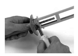
• Slide the I.D. steel onto the I.D. steel rod. Slide a spring onto the I.D. steel rod. Install and tighten the I.D. steel screw.
