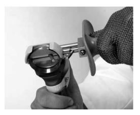
• While holding the Bettcher<sup>®</sup> E-Z EDGE Sharpening device locator down firmly on the trimmer blade housing, push the sharpening rod toward the trimmer blade. Hold the sharpening rod against the outside blade edge for a few seconds, with very light pressure applied. This sharpens the outside edge of the blade.
