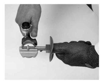
Note: The forward and backward motion need only be performed once to sharpen and steel the blade's edge.
