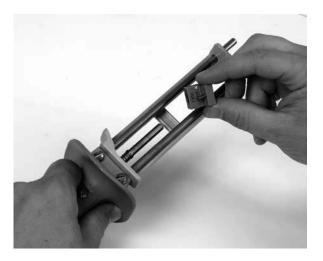
• Remove the I.D. steel rod screw. Then remove the I.D. steel rod.
