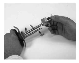
• Remove the steeling rod screw from the rod mount and remove the steeling rod shaft.
