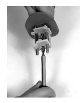
• Remove the spring rod screw, then remove the spring rod, I.D. steel, spring, and locator.
