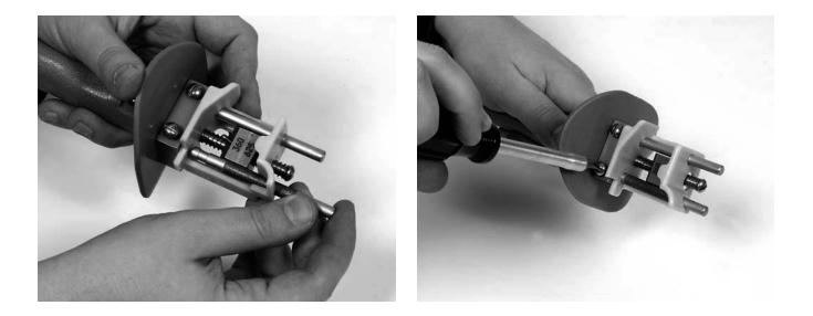
• The locator and I.D. steel should move freely on their rods.
