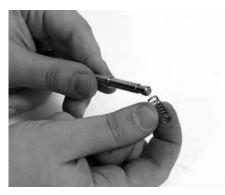
• Slide the I.D. steel rod with spring through the locator and into the rod mount. Tighten the I.D. steel rod screw.
