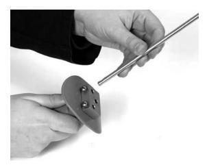
• Remove the handle screw and pull the rod mount out of the handle.
