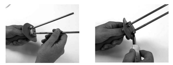
• Slide the locator on to the sharpening and steeling rods with the three smallest holes against the rod mount.
