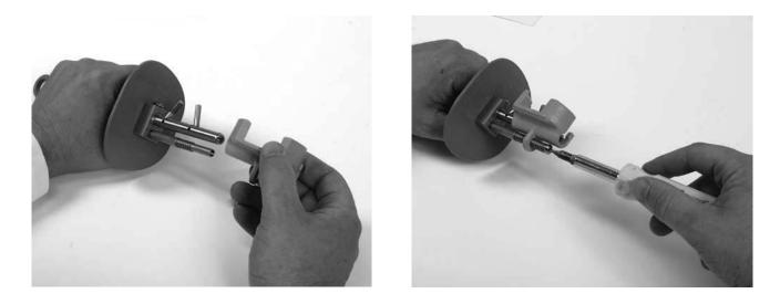
• Ensure the locator moves freely back and forth on the rods.
