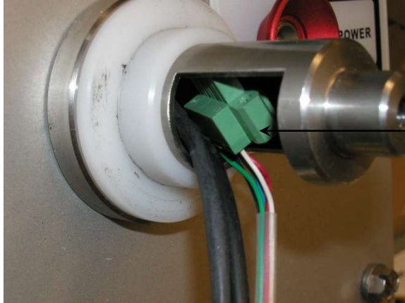
Plugs Fed Through the Hollow Opening in the Pivot Post
