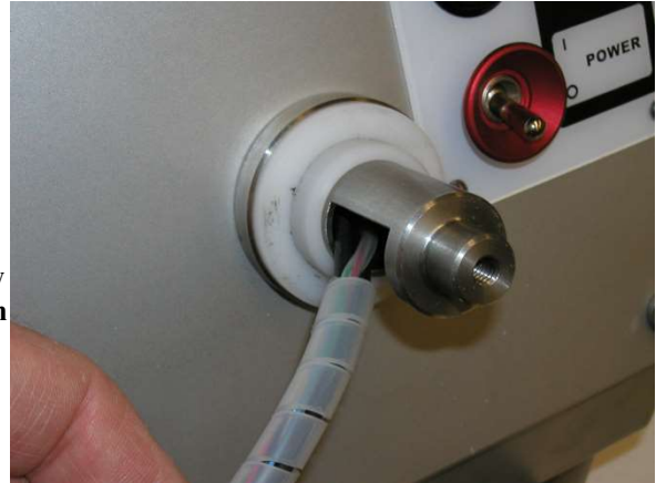
Plugs Fed Through the Hollow Opening in the Pivot Post
