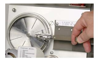
• Move the Steeling Arm so the front Guide Pins come out of the Steeling Device Slide then lift the Steeling Arm up and pivot it on the Rear Guide Pins so the Steeling Arm rests on the Steeling Slide Body.
