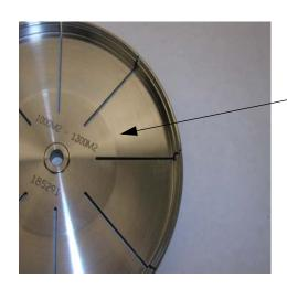
The Blade Model(s) and the Blade Holder Part Number are Etched on the Holder.
