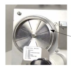
Blade Installed in Blade Holder.
