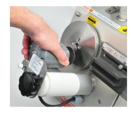
Rotate Motor Counterclockwise.
