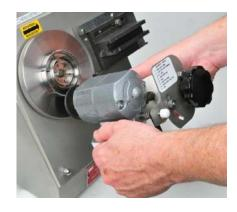
Grasp the Motor Pivot and Rotate Clockwise Against the Blade.
