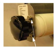
Loosen Screws to Rotate the Grinder Motor, Motor Pivot and Position Plate.
