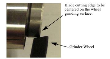
If the blade and Grinder Wheel do not make contact as shown, loosen the two screws on the Position Plate and rotate the Grinder Motor, Motor Pivot and Position Plate as a unit until the blade to wheel contact is as shown.
