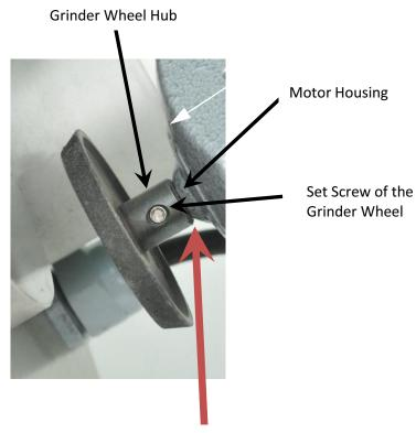
1/64 inch (4mm) space between the end of the Grinder Wheel Hub and the front of the Motor Housing.
