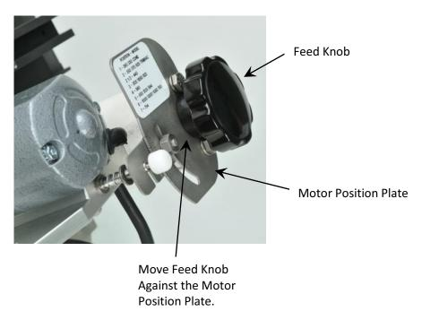
• Turn the Feed Knob Counterclockwise to move the Grinder Motor to its full back position.
