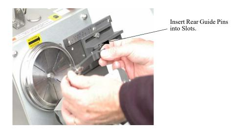
• Move the Steeling Arm to the right until the front Guide Pins align with the slots then lower the Steeling Arm into the Steeling Device Slide.
