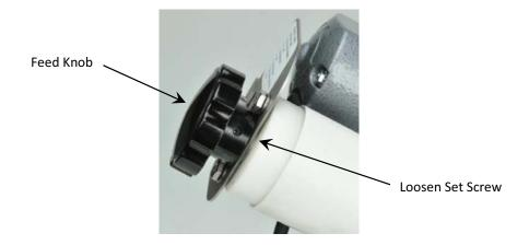
• With the Set Screw still loosened, turn the Feed Knob **Clockwise**, running the Grinder Motor in toward the Blade Holder to within 1/64 inch (.4mm) from the top of the Blade Holder.
