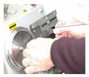
Align Front Guide Pins to Slots and Lower Steeling Arm into the Steeling Device Slide.
