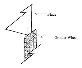
If the blade and wheel do not make contact, loosen the two screws under the pedestal knob and rotate the grinder, motor pivot and positioner plate as a unit until the blade to wheel contact is as shown. Should more adjustment be needed, loosen the pedestal mounting screws on the rear side of the base plate. Then rotate the pedestal assembly as a unit until the blade and grinder wheel make contact and tighten all screws.
