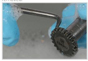
**5. Rinse and Dry:** Be sure all parts are completely dry. Using compressed air is highly recommended.
