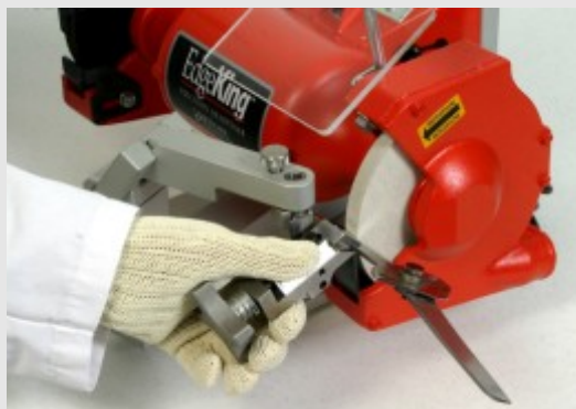
Buffing the blade removes the burr.
