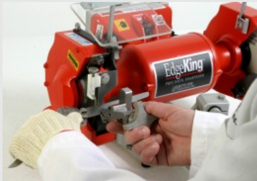
Grind the blade to return the edge.
