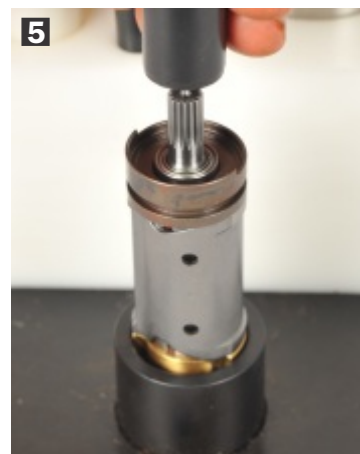
5 Using the bearing tool and hammer, tap bearing onto cylinder. Make sure notches are aligned (note circle).
