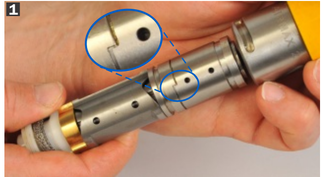
1 Align the power components and push up inside the AirMax™ handle.
