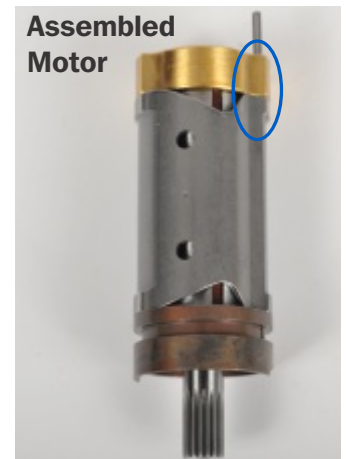
5 Using the bearing tool and hammer, tap bearing onto cylinder. Make sure notches are aligned (note circle).
