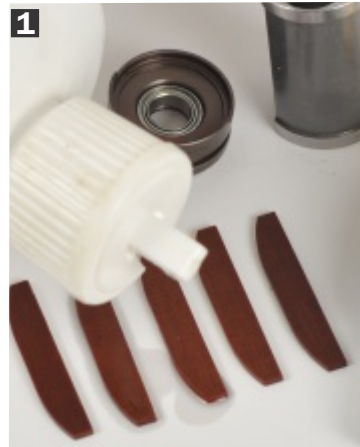
1 Saturate vanes and insert in rotor, curved side towards rotor.
