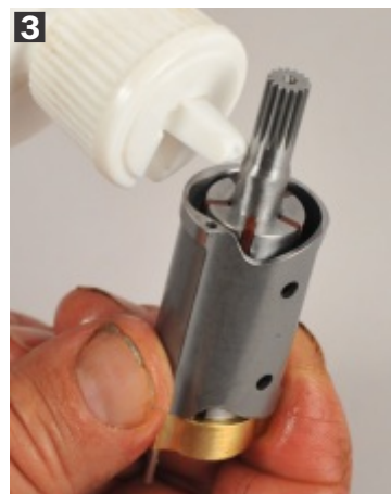
3 Add a small amount of Whizard® Oil and then place in the maintenance tool block.
