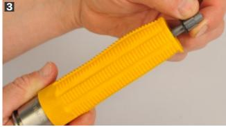
Using the driver adapter, rotate the air motor back and forth.
