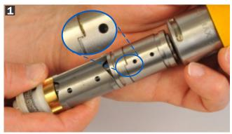
Align the power components and push up inside the AirMax  $^{\rm \tiny M}$  handle.
