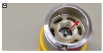
When the air motor is properly installed there will be one or two threads visible — too many or no threads means miss installation.
