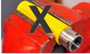
Never put the AirMax<sup>™</sup> handle into a vice, this will crush the hollow handle.
