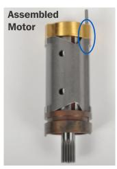
Using the bearing tool and hammer, tap bearing onto cylinder. Make sure notches are aligned (note circle).
