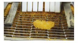
**Good Vibrations** – The ingenious vibrator springs shake off excess breading – saving on ingredient costs and extending oil life.
