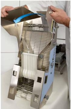
New split breading conveyor is easier to lift – and it separates for ease of cleaning.
